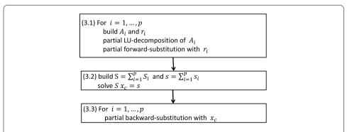
**Figure 3 Steps to build and solve the BBD system.** This figure illustrates in more detail steps (1.4) and (1.5) of the inner loop in Figure 1 in the frame of our BBD approach. Both of the loops, step (3.1) and step (3.3) of this figure can be done in fully parallel and decoupled mode, whereas step (3.2) represents the sequential bottleneck of the BBD approach.
