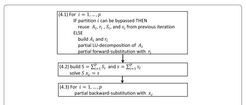
Figure 4 Partition bypass acceleration. If the bypass criterion for a partition is met, the devices within this partition need not to be evaluated and matrix LU-decomposition can also be skipped. Subsequent computations are unchanged compared to Figure 3.
