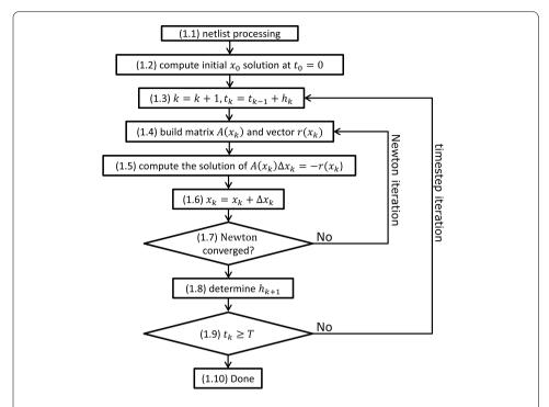
**Figure 1 Transient analysis algorithm.** The flow diagram presents the algorithmic steps during the transient analysis. The steps (1.4)-(1.7) within the nested loop are the most critical in the transient analysis. The outer loop represents the time loop of the whole circuit.
