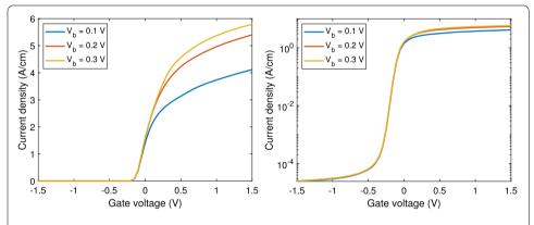
Figure 3 Characteristic curves of the simulated GFET in linear scale (left) and logarithmic one (right). The adopted model is (1), (4)
