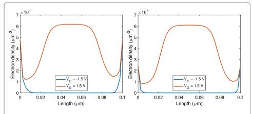
Figure 4 Electron density of the simulated GFET in the case  $V_b = 0.2$  V and  $V_G = -1.5$  and 1.5 V. On the left the adopted model is (1), (2); on the right it is (1), (4)
