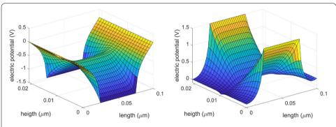
Figure 6 Electrostatic potential of the simulated GFET in the case  $V_b = 0.2$  V and  $V_G = -1.5$  V (left) and  $V_G = 1.5$  V (right)
