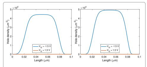
Figure 5 Hole density of the simulated GFET in the case  $V_b = 0.2$  V and  $V_G = -1.5$  and 1.5 V. On the left the adopted model is (1), (2); on the right it is (1), (4)
