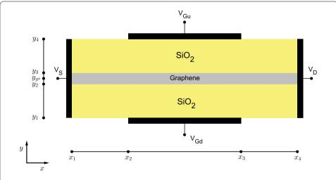
**Figure 1** Schematic representation of the simulated GFET. In the direction orthogonal to the *xy*-plane the device is assumed infinitely long
