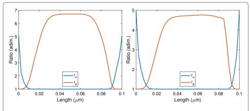
**Figure 7** Ratios of the degenerate and non-degenerate diffusion coefficients in the case  $V_b = 0.2$  V and  $V_G = -1.5$  V (left) and  $V_G = 1.5$  V (right)
